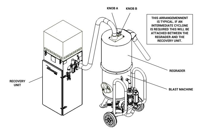
IMPORTANT NOTICE: THE INLET DAMPERS ON THE CYCLONE SHOULD BE IN THE FULLY OPEN POSITION FOR MOST COMMON ABRASIVE TYPES AND GRADES. THESE DAMPERS ENABLE MORE FINITE SEPARATION TO BE ACHIEVED WHEN FINE GRADES OF LIGHTER MATERIAL IS BEING RECYCLED
